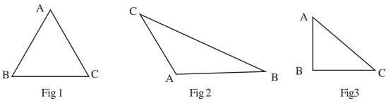
Obtuse Angled Triangle **Fig 2**: A line segment AB is drawn. At one end say A, an obtuse angle(>90<sup> $\circ$ </sup> &<180<sup> $\circ$ </sup>) is drawn with the help of a protractor. The second line attached to the angle is AC. On joining BC we get an obtuse angled triangle. Here angle CAB>90<sup> $\circ$ </sup> but <180<sup> $\circ$ </sup>
